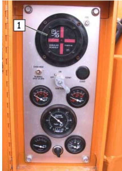
Fig. 3-6 Instrument Panel - Cummins Engine 1. Vertical Indicator Digital Readout
