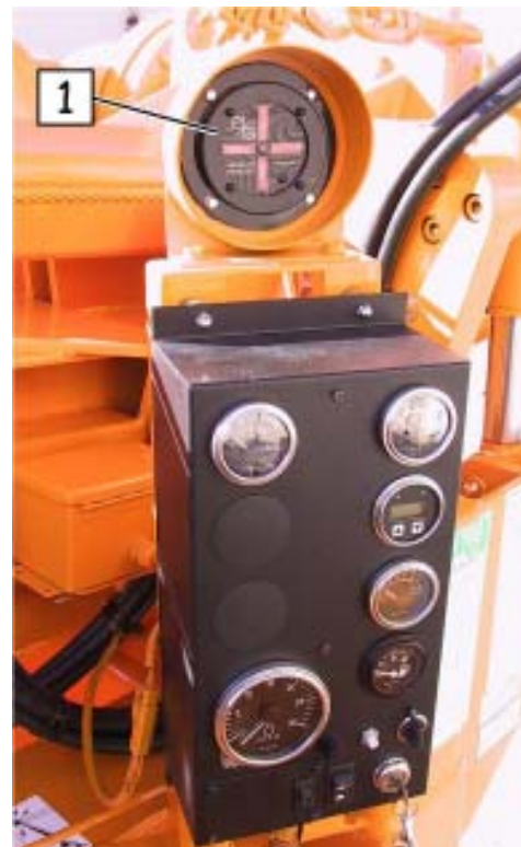
Fig. 3-6a Instrument Panel - John Deere Engine 1. Vertical Indicator Digital Readout
