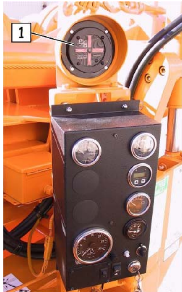
Fig. 4-4 Instrument Panel - John Deere Engine 1. Vertical Indicator Digital Readout
