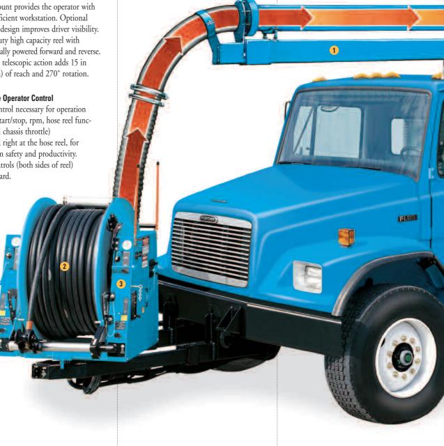
Vactor® 2100 Series Positive Displacement Sewer Cleaner
